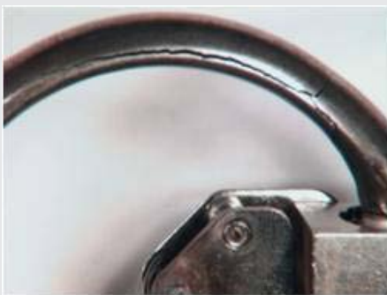
Picture: fractured Bourdon tube
